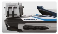
Rear Deck Extension with LinQ attachment system Adds 29 cm to the back of the watercraft to increase stability, space, and storage capability.
